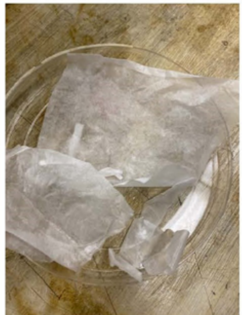
Figure 3. Separated and dried plastic liner of a single cup
