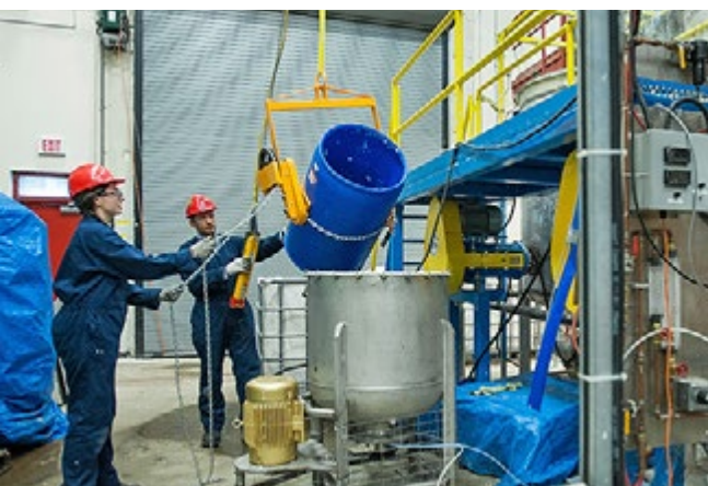
Above: Nici Darychuk and Francisco Fernandez handle pulp suspension in preparation for a pilot scale energy reduction experiment. Photo: Martin Dee
