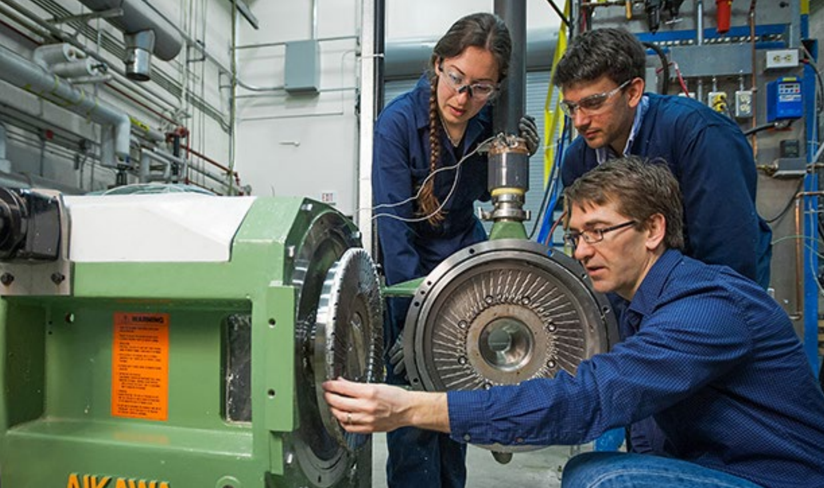
Above: James Olson, Francisco Fernandez and Nici Darychuk examine an experimental refiner plate on the PPC's low consistency refiner Photo: Martin Dee
