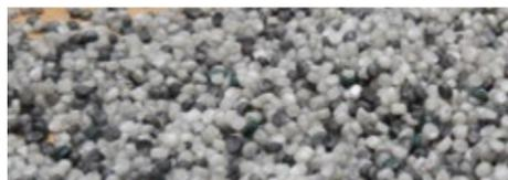
Left: A mixture of magnetic (black) and non-magnetic (white) high density polyethylenes (PE). The current study involves PE's with different colors that are employed in an investigation of particles intermixing in a dual-slot rectangular spouted bed. These different colors' PE's have the same physical properties. Effects of gas velocity, static bed height, and slot width are experimentally investigated.
