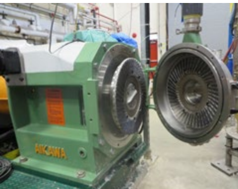
Pictured: Low Consistency Refiner donated by AIKAWA/Advanced Fibre Technologies Inc. The state-of-the-art equipment is an ideal size for industry focused, university research. It is large enough to reproduce industrial refining performance while being small enough to enable relatively small amounts of pulp to be used.
